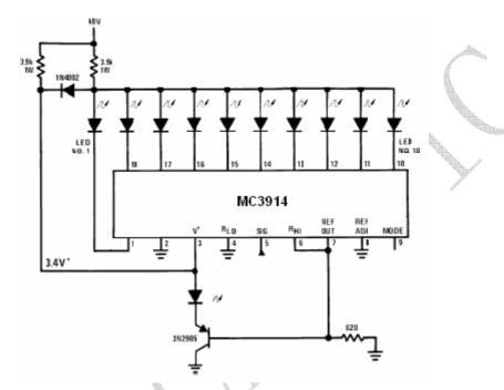
The LED currents are approximately 10 mA, and the MC3914 outputs operate in saturation for minimum dissipation.
