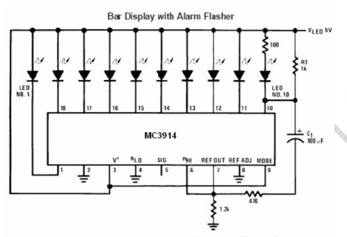
Full-scale causes the full bar display to flash. If the junction of R1 and C1 is connected to a different LED cathode, the display will flash when that LED lights, and at any higher input signal.
