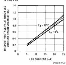
LED Driver Saturation Voltage
