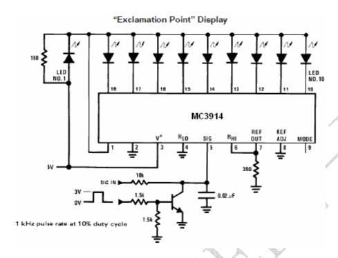
LEDs light up as illustrated with the upper lit LED indicating the actual input voltage. The display appears to increase resolution and provides an analog indication of overrange.
