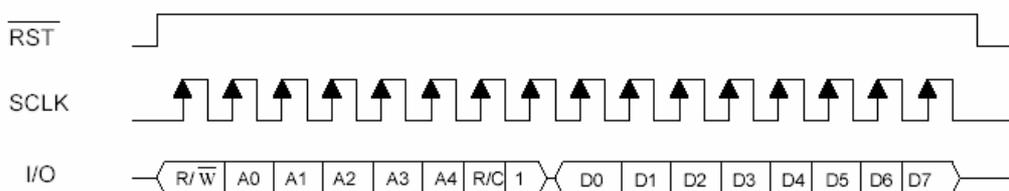
In burst mode,  $\overline{RST}$  is kept high and additional SCLK cycles are sent until the end of the burst.
